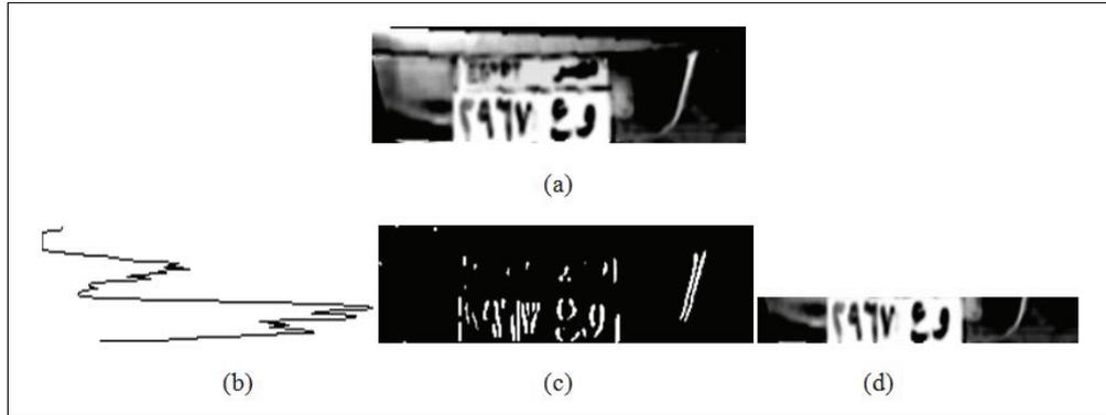
FIGURE 6. (a) an image after before the step of cutting top and bottom extra parts; (b) the vertical projection of image (c); (c) Sobel vertical edge detection for image (a); (d) the exact band of the plate after cutting the top and bottom extra parts
