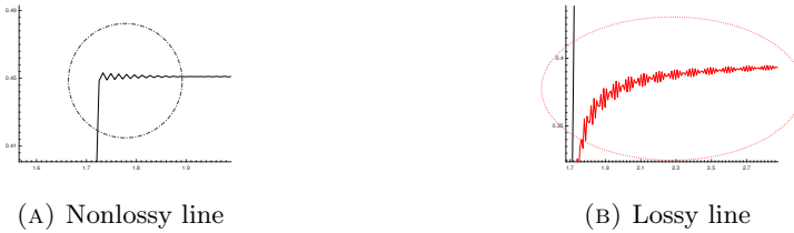
FIGURE 3. Leading edge of the load voltage by FDTD for nonlossy line (A) and lossy line (B).
