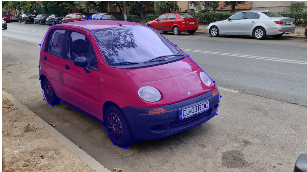
FIGURE 3. Blue polygon that defines the ROI for the Matiz class. Each point from the label file is marked with a filled circle for easier visualization.
