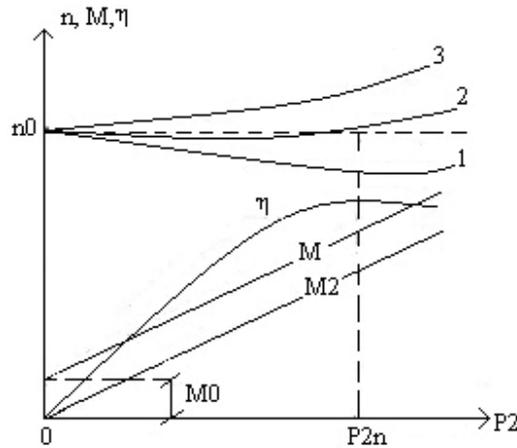
FIGURE 1. The operating characteristics of DC motor with excitation derivation
