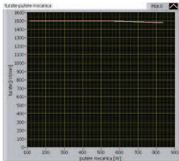
FIGURE 9. The operation characteristic represented by the speed according to the mechanic power
