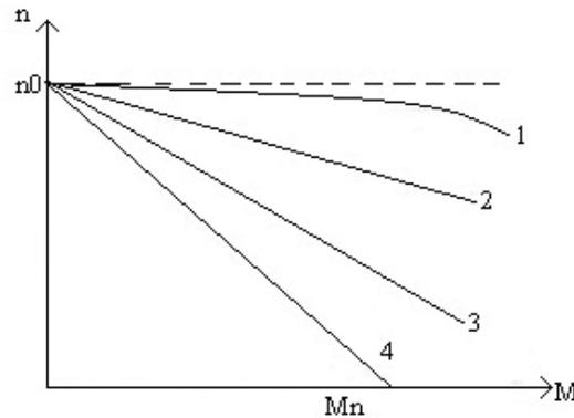
FIGURE 2. The mechanical characteristics of the direct current engine with excitation derivation
