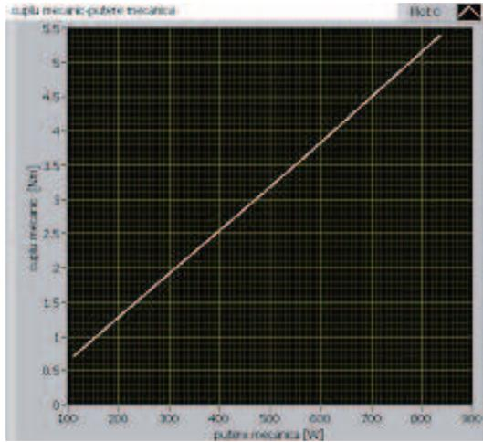
FIGURE 10. The operation characteristic represented by the mechanic torque according to the mechanic power
