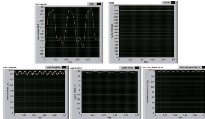
FIGURE 6. The front panel of the virtual instrument achieved for the acquisition of the measures necessary to the increase of the operation characteristics of the direct current engine with excitation derivation
