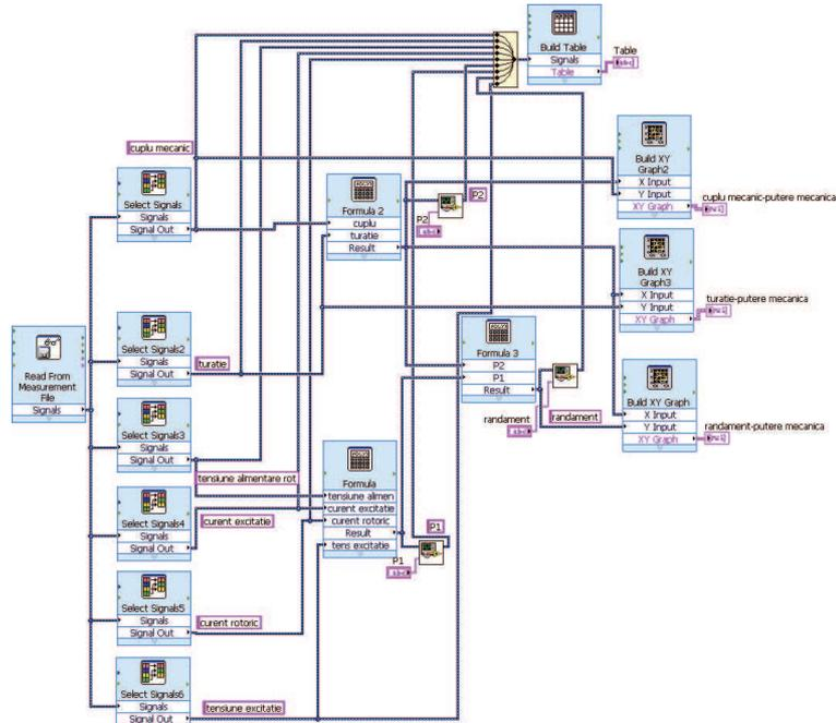
FIGURE 7. The block diagram of the virtual instrument achieved for the determination of the operation characteristics of the direct current engine
