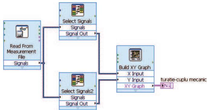
FIGURE 12. The block diagram of the virtual instrument achieved for determining the mechanical characteristic
