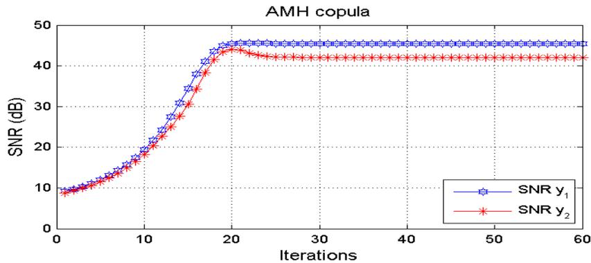
FIGURE 4. Average output SNRs versus iteration number : Uniform dependent sources from AMH-copula.
