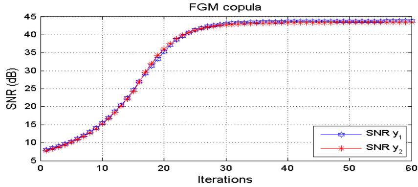
FIGURE 5. Average output SNRs versus iteration number : Bpsk dependent sources from FGM-copula.
