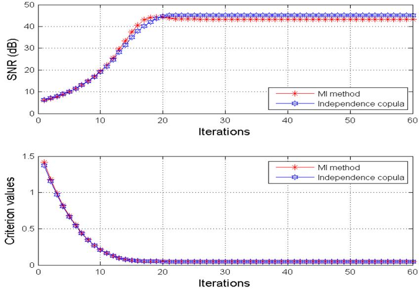
FIGURE 10. Average output SNRs versus iteration number: uniform independent sources.
