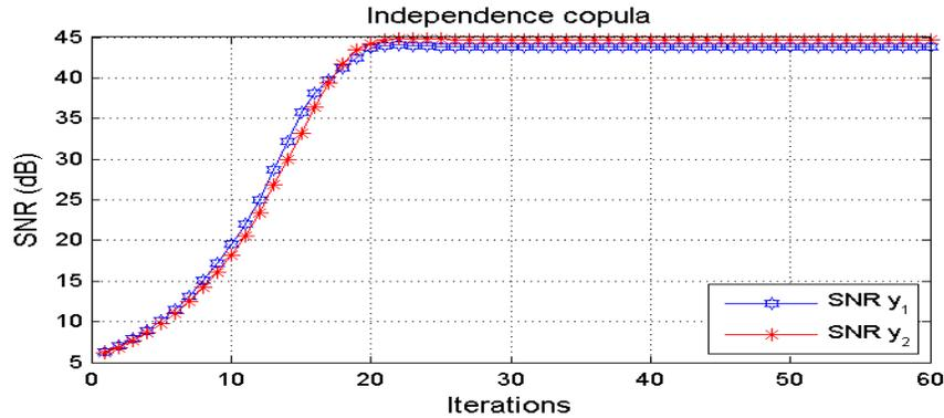
FIGURE 2. Average output SNRs versus iteration number : ASK independent sources.
