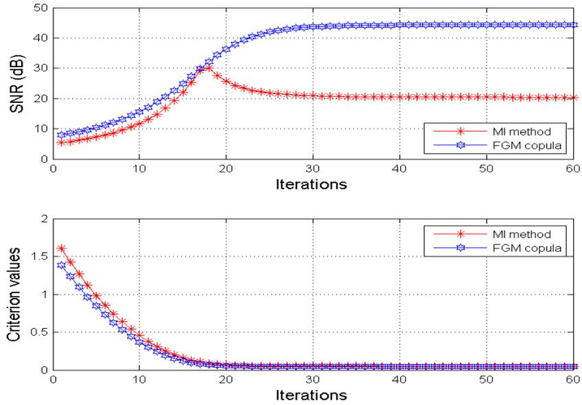
FIGURE 11. Average output SNRs versus iteration number: BPSK dependent sources from FGM-copula.
