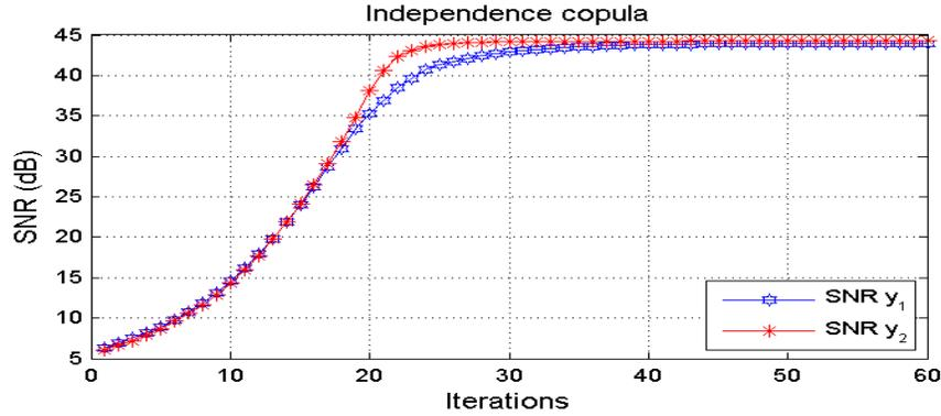
FIGURE 1. Average output SNRs versus iteration number : Uniform independent sources.
