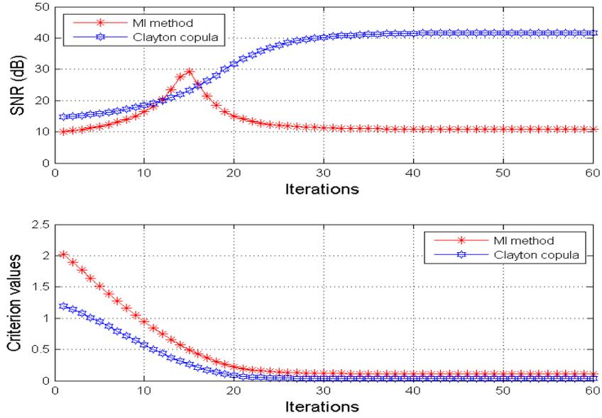
FIGURE 12. Average output SNRs versus iteration number: uniform dependent sources from Clayton-copula.
